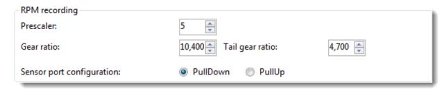
The field *Prescaler* sets how many pulses per revolution of the engine the rpm sensor puts out. For electrical engines this is mainly the count of the poles **pairs**. So with a 10 pole engine you would have to enter "5" here.
