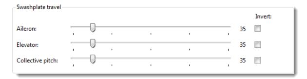
With the settings in *Swashplate travel* the cyclic throws for aileron, elevator and collective pitch can be adjusted.
